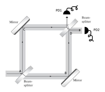
Suppose the optical path length (not including phase shifts due to reflection) is exactly equal for legs 1 and 2. Also suppose that the intensity of the laser before the MZI is  $I_0$ , and the light is in a very narrow beam.
