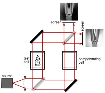
Figure caption (from Wikipedia): The Mach–Zehnder interferometer is frequently used in the fields of aerodynamics, plasma physics and heat transfer to measure pressure, density, and temperature changes in gases. In this figure, we imagine analyzing a candle flame. Either output image may be monitored. Credit: Wikipedia, Stigmatella aurantiaca with modification by Kid222r
